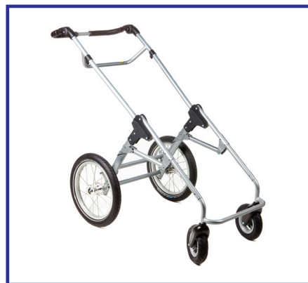
Frame with two 16" rear wheels, two 10" swivel wheels, and park brake.
